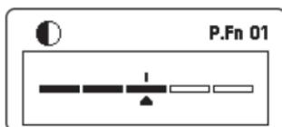
You can adjust the contrast of the LCD panel in 5 levels.
