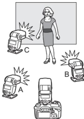
You can add firing group C to firing groups A and B. C is convenient to set lighting so as to eliminate the subject's shadow.
