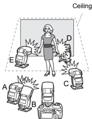
When using an EOS DIGITAL camera released in and after 2012, such as the EOS-1D X, you can shoot in a different flash mode set for each firing group with up to 5 groups (A, B, C, D, and E).
